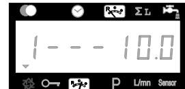
The valve is in cycle 1, 10 min is remaining in that cycle.
