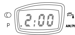
Regeneration time For example: 2 A.M. (only visualised in delayed metered and timeclock mode)
