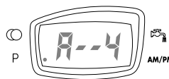
Day override (maximum days between 2 regenerations) For Example : regeneration every 4 days (only visualised in timeclock mode, setting is imperative.)
